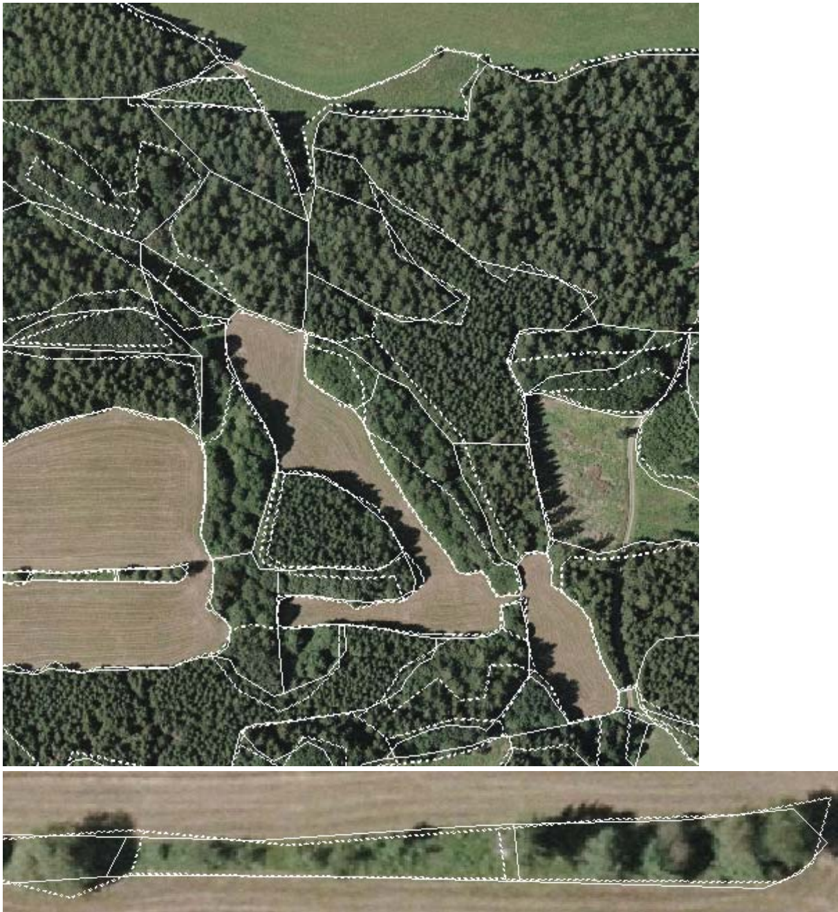
Fig. 1: Vectorization of boundaries of the categories used in CzechTerra, carried out independently by two experienced operators (the two versions are shown in full line and in dotted line). The course of the boundaries is very different, especially in the forest. In elements which are easily identified (here, a field margin in agricultural grassland), the course of the boundaries is similar, but sliver polygons would occur in an overlay analysis.
